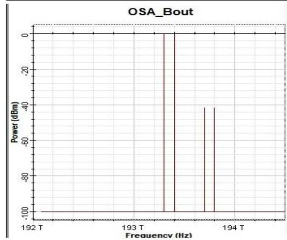
Fig. 5: Output at OADM-A & B for flow 1
