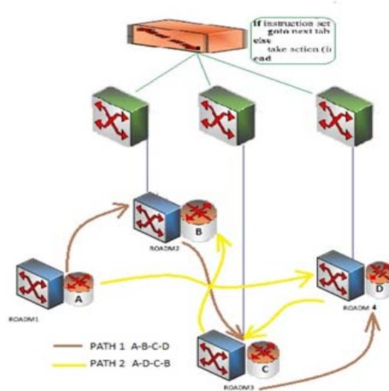
Fig. 2: Design showing control and data planes
