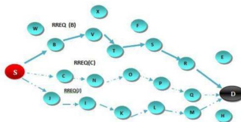
Figure 4 : Route Discovery Procedures in AOMDV
