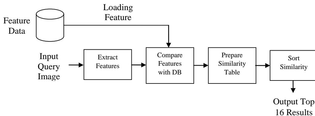
Figure 3.2 : Block Diagram of Image Retrieval
