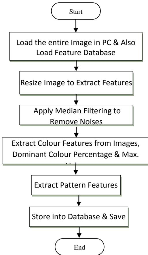
Figure 3.3 : Flow char of feature database preparation
