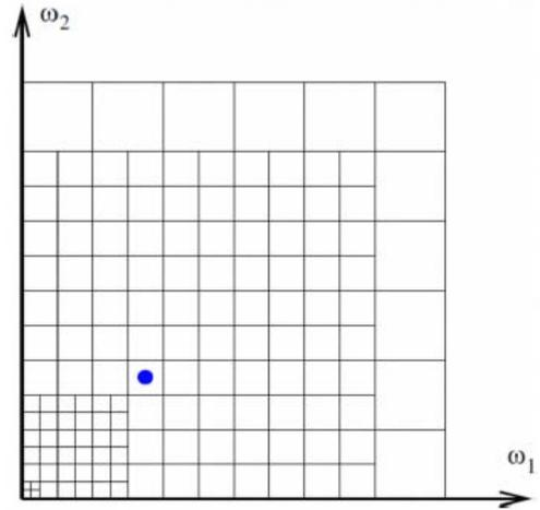
Figure 5 : Wave atom tiling of the frequency plane
