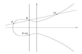
Fig.2: Adding two points on elliptic curve
