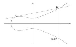
Fig.3 : Doubling a point on an elliptic curve
