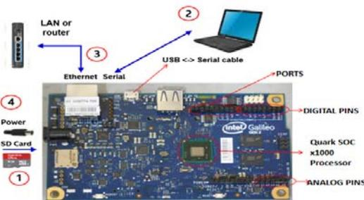
Figure 4 : Intel Galileo Gen2 Development Board [8]
