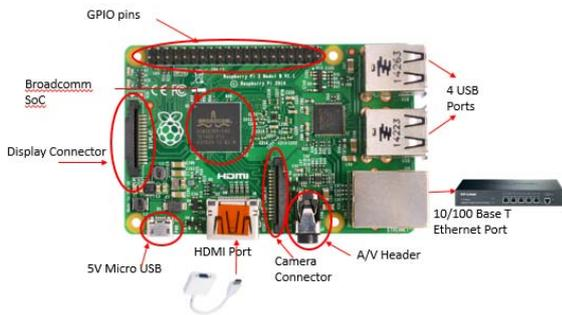
Figure 3 : Raspberry Pi2 Development Board [7]
