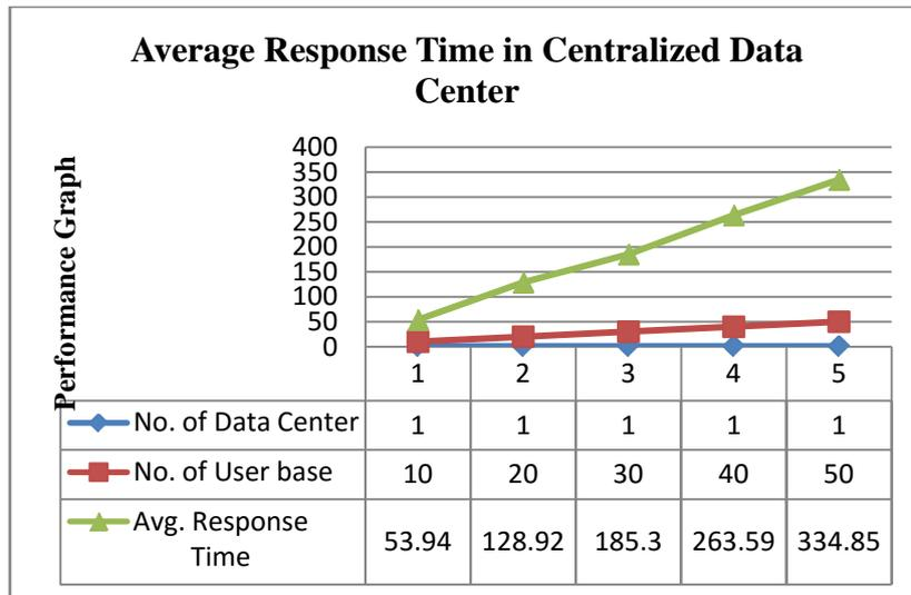
Figure 4: Performance graph in terms of response time of Centralized Data Center
