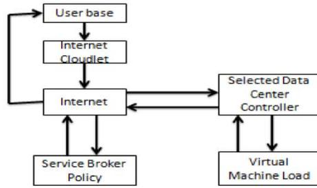
Figure 3: User Request Routing in Cloud Analyst
