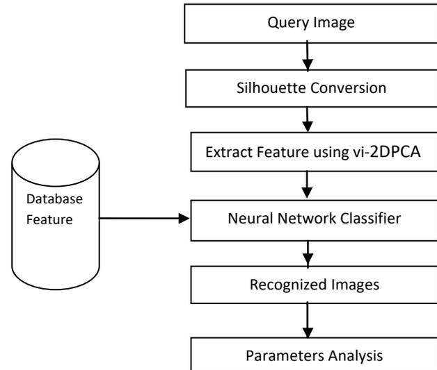
Step1. In this processing, different frames from video has been extracted and these frames have been used for silhouette conversion by removing back ground from the frames of the video and these frames have been used for silhouette conversion by removing back ground from the frames of the video.
