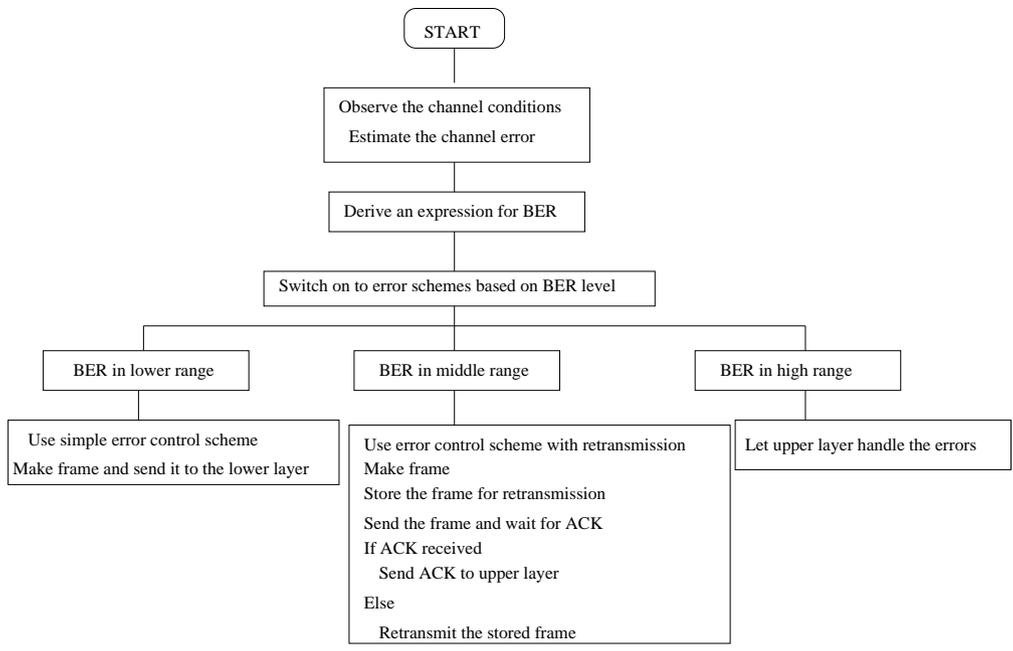
Figure 1: Channel adaptive error control scheme
