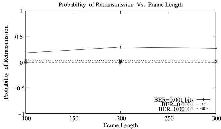
Figure 8: Probability of Retransmission Vs. Frame lengths for different BERs
