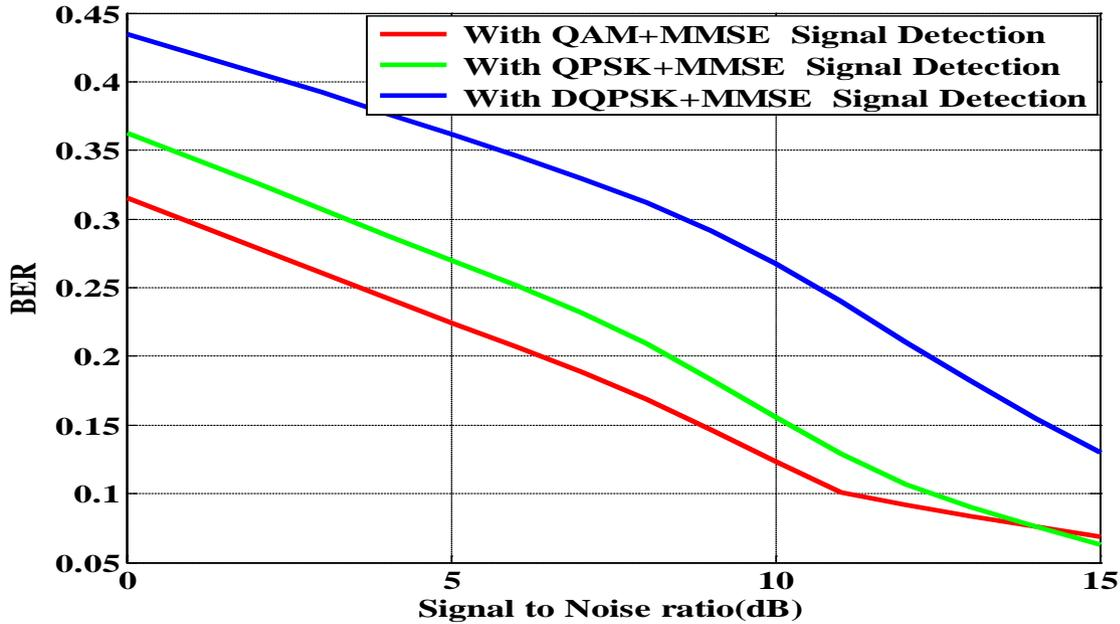
Figure 2: BER performance of LDPC channel encoded MP-WFRFT based Physical Layer Security Scheme implemented MIMO wireless communication under utilization of various digital modulation and MMSE signal detection technique
