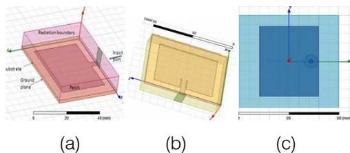
Fig. 4: Microstrip Direct feed (a) Inset Feed (b) Coaxial Feed [20].
