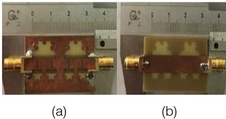
Fig. 10: Fabricated Koch FDGS with 2 cascaded resonators. (a) Bottom side (DGS). (b) Top side (microstrip transmission line) [41].
