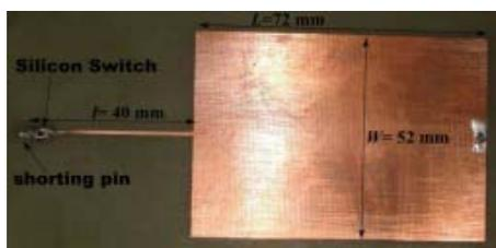
Fig. 8: Optically shorted stub-loaded frequency-switching patch antenna [29].
