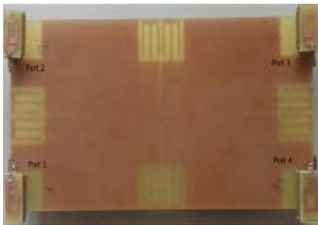
Fig. 1: Multiband MIMO with Insertion of parasitic element [9].
