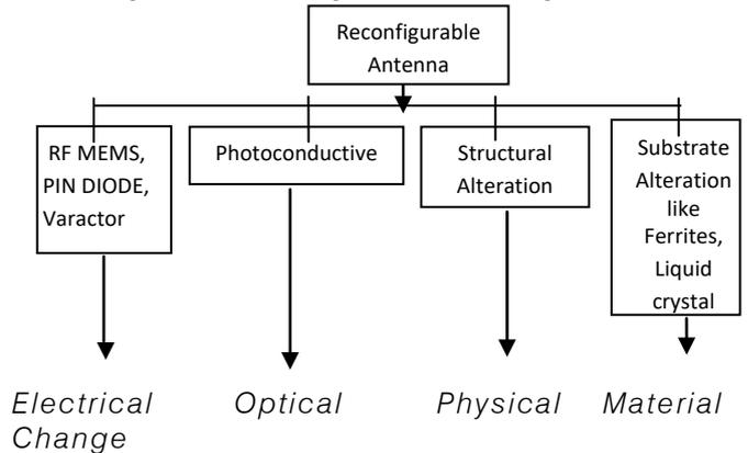
Fig. 6: Reconfigurable antenna various techniques.
