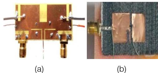
Fig. 7: (a) Antenna with MEMS switches [26] (b) reconfigurable antenna using PIN diode [27].
