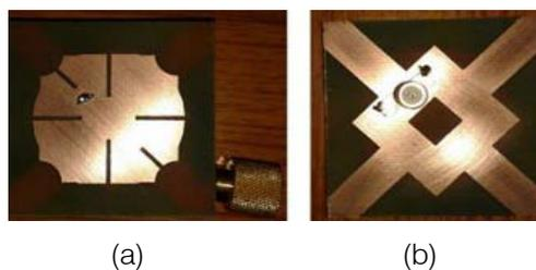
Fig. 9: Multiband Compact CP Antenna with DGS [34].
