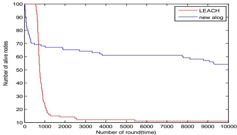
Figure 4 : Comparative analysis of LEACH and new protocol
