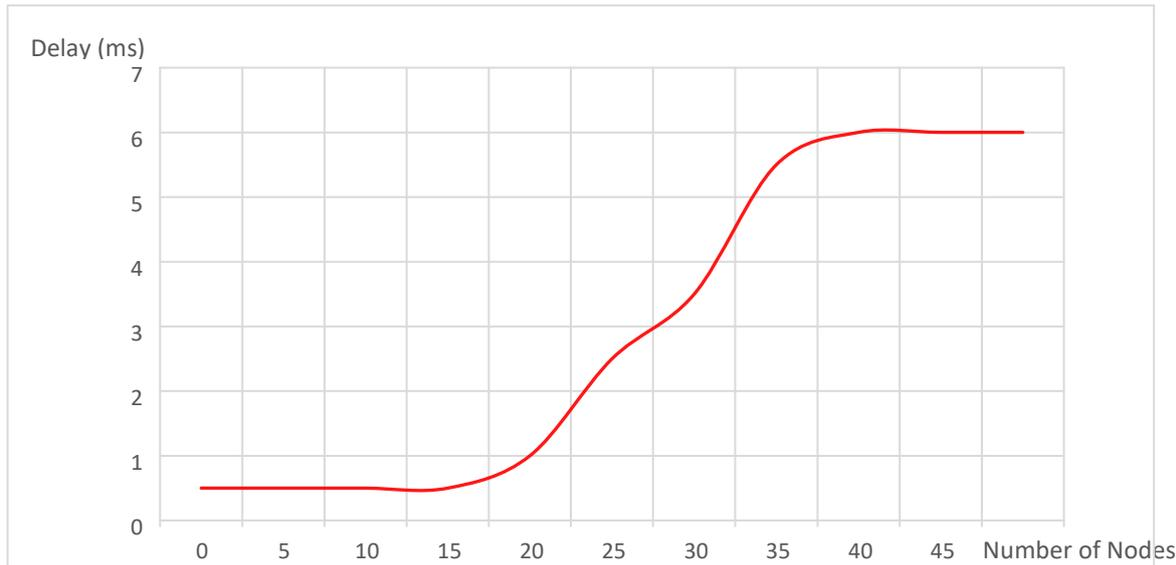
Figure 6: Average End-to-End Delay Analysis of Simulated Long-Term Evolution Network Environment
