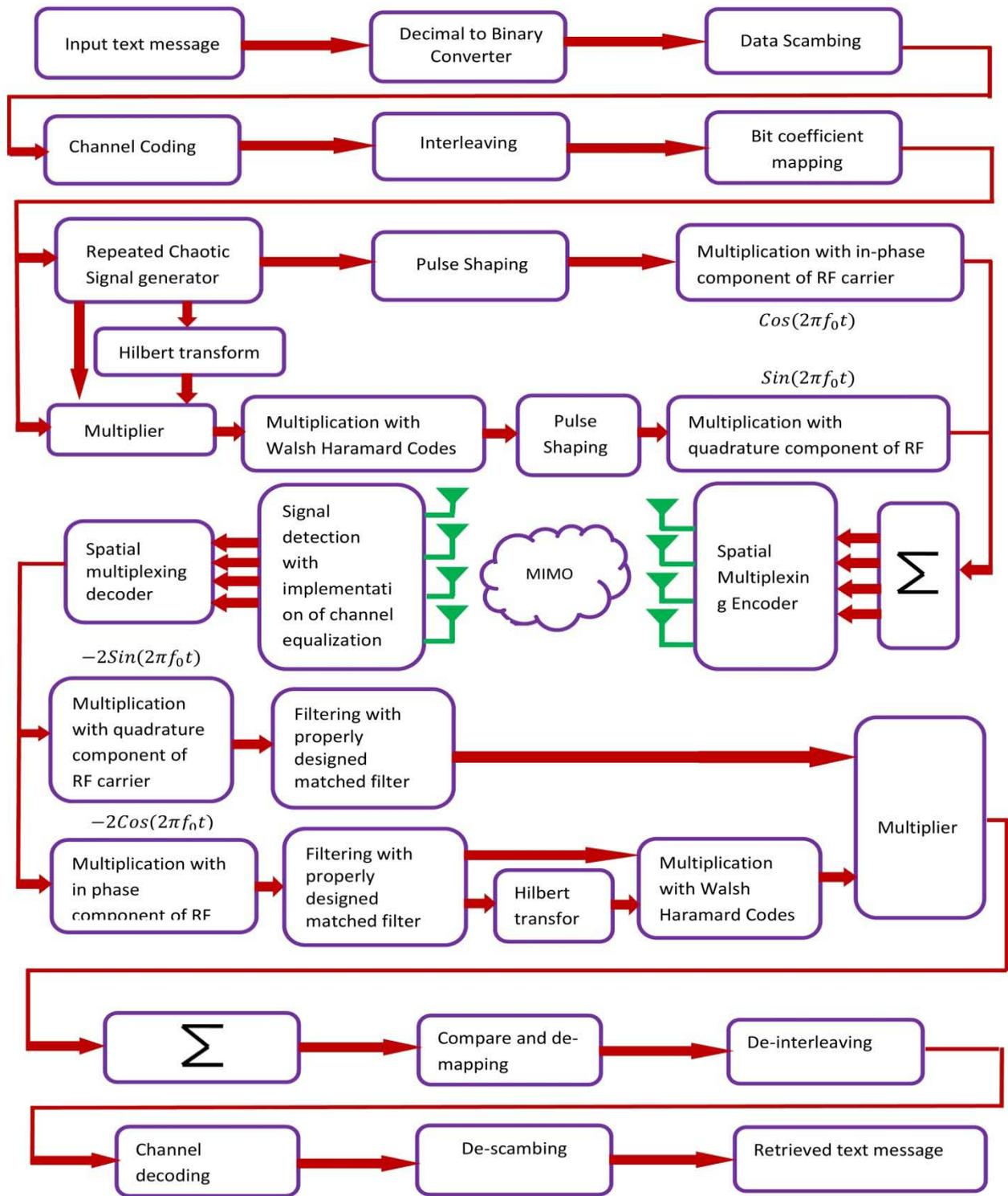
Fig.1: Block diagram of Encrypted text message transmission in 5G compatible Orthogonal Multi-level Chaos Shift Keying Modulation Scheme Aided MIMO Wireless Communication System
