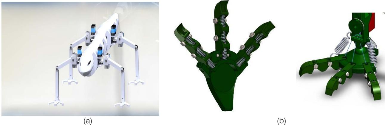
Fig. 4: Mobile robot a lizard analog
