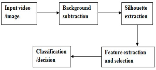
Figure 1: General Block diagram of a gait recognition system
