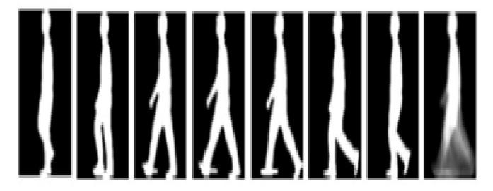
*Figure 3:* Normalized and aligned images. The last image corresponds to Gait Energy Image [8]
