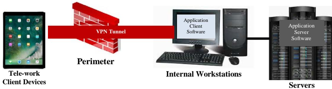
Figure 5: Direct Application Access Architecture
