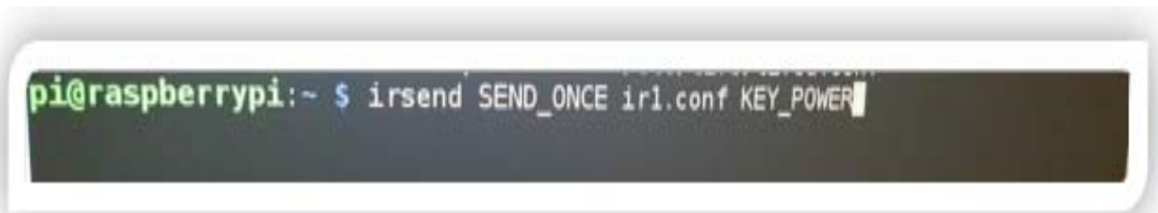
Figure 26: Screenshot of switching air conditioner in command window
