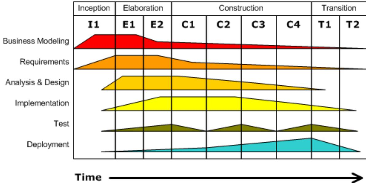
Figure 7: UP lifecycle (Source: Wikipedia at [http://en.wikipedia.org/wiki/Unified\\_Process](http://en.wikipedia.org/wiki/Unified_Process))
