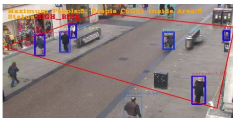
Fig. 6: Final output of Density Risk detection
