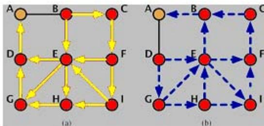
Figure 2 : Illustration of node-independent trees for the example network. (a) Red tree. (b) Blue tree. Node A is the root (destination) node
