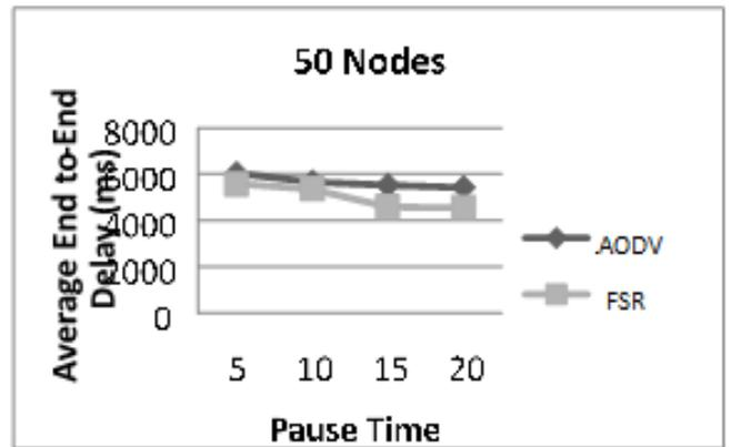
Figure 2(b) : Average End-to-End Delay for 50 Nodes
