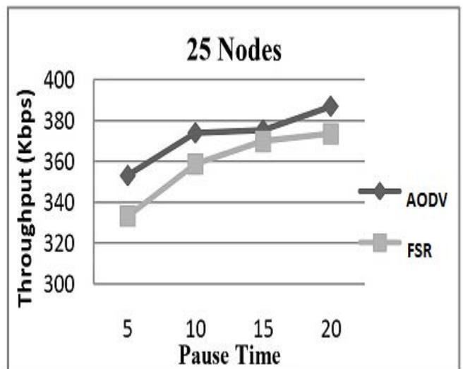
Figure 1(a) : Throughput for 25 nodes
