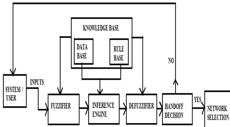
Figure 2 : Block Diagram for Vertical Handoff Decision
