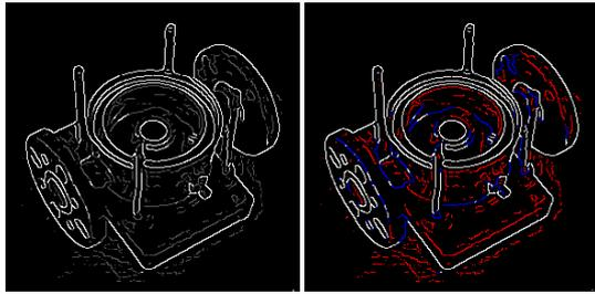
(e) Double thresholding (f) Edge tracking by hysteresis
