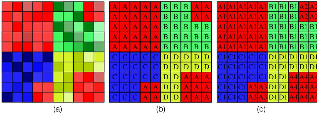
Fig.2: Schematic diagram of the result of ANN cloud classification and ANN-SRG segmentation
