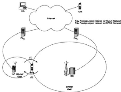
Figure2- Proposed IP-based handoff architecture.
