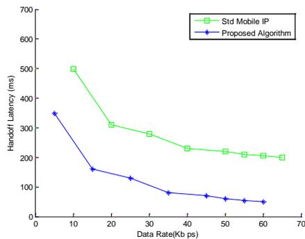
Figure 5. Comparison of handoff latency for different data rates. Standard mobile IP versus proposed algorithm.
