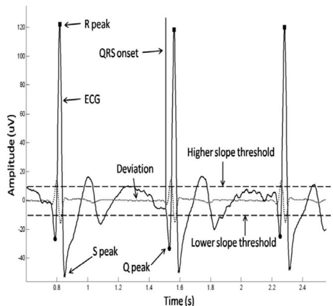
Fig.3 : QRS Detection of the Normal ECG Waves
