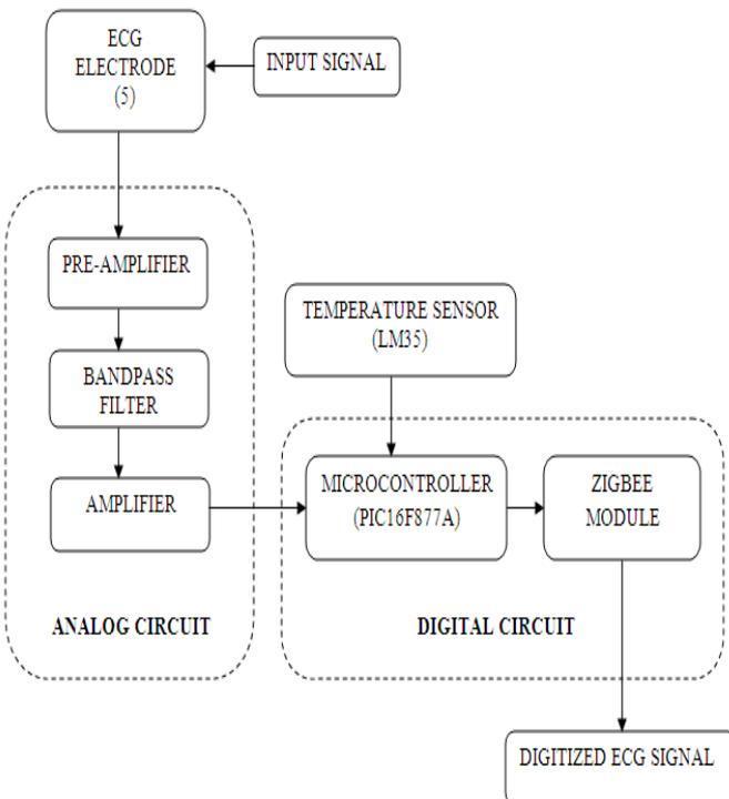
Fig.2 : Block Diagram of ECG Device
