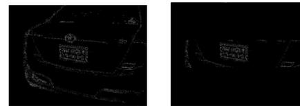
Fig.2 : (a) Sobel vertical edge detection (b) Effect of threshold
