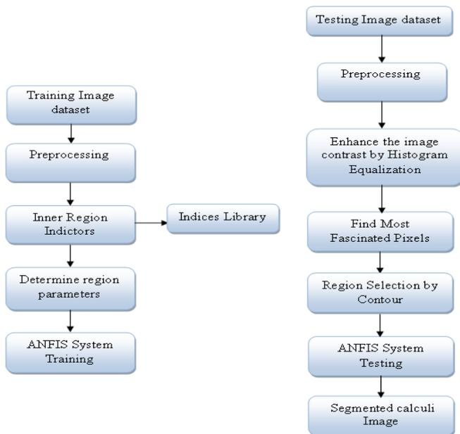
Fig. 1. Proposed RICS segmentation training and testing procedure
