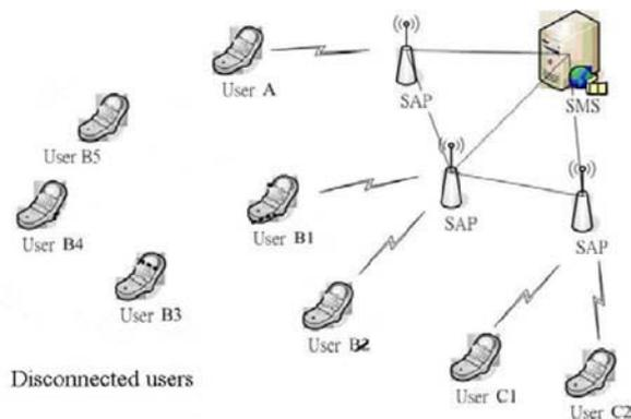
Fig 3.1 : System architecture for mobile streaming service
