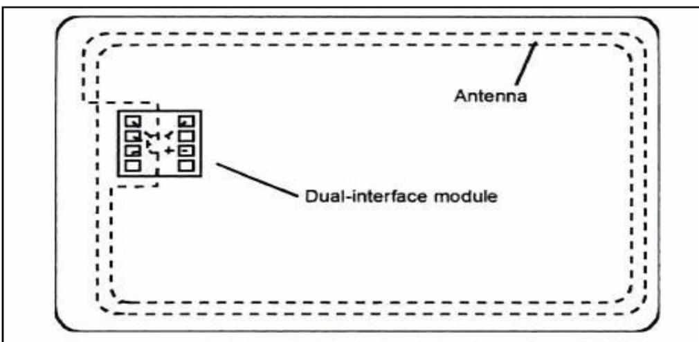
Figure 6: Schematic of smart card without contact
