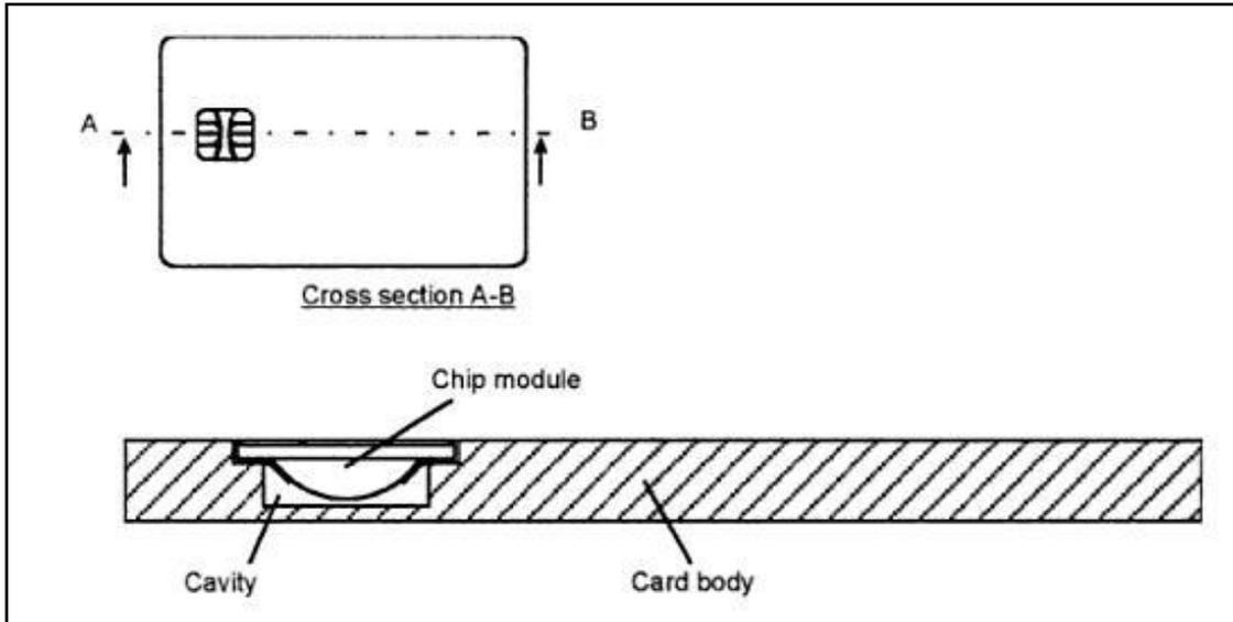
Figure 5: Schematic of Contact smart card
