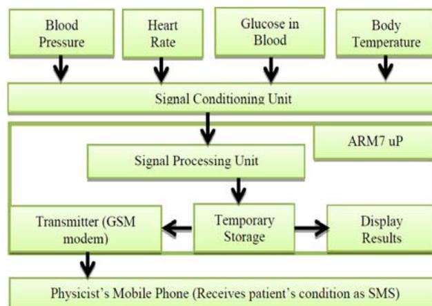
Figure 1 : Complete block diagram of the proposed system
