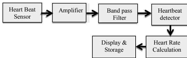
Figure 3 : Generalized block diagram for heart rate monitoring
