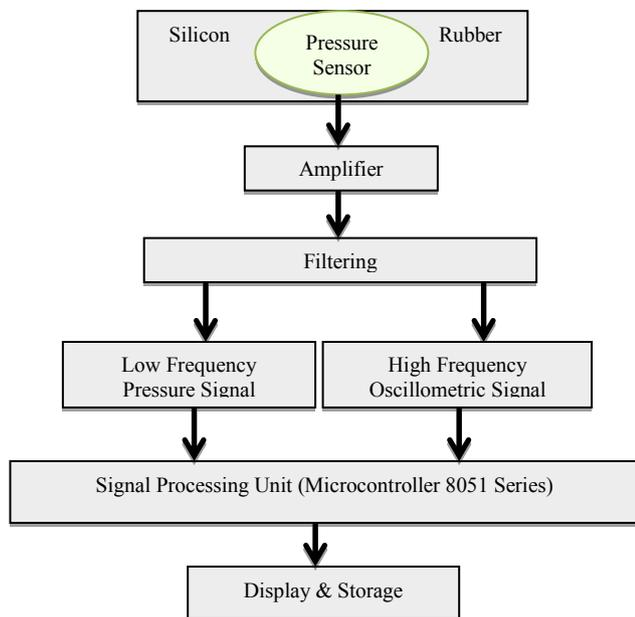
Figure 2 : Cuffless Blood Pressure Measuring System
