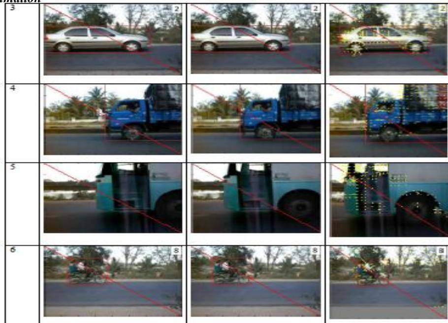
**Fig.2-Display of results of optical flow needle diagram for different vehicles**
