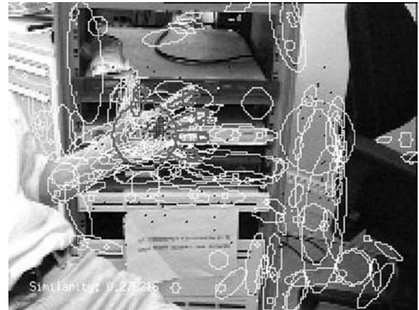
Fig. 3 : Detected multi-scale features and the recognized hand pose superimposed in an image of a complex scene.
