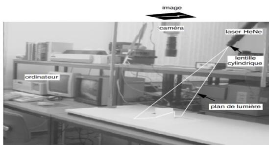
Fig. 2 : Experimental system for range image acquisition
