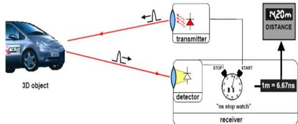
Fig. 3 : Flight time system for range image acquisition
